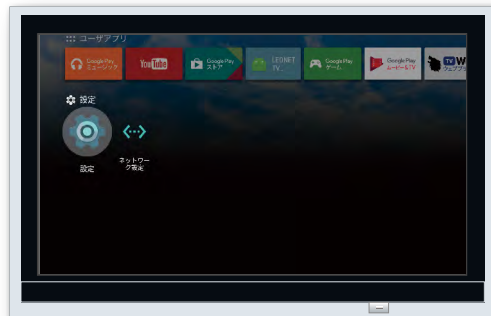
Scroll down to select Settings and press OK on the remote control.
